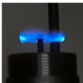
"Crown" flame when burning hexane
