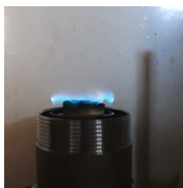
"Crown" flame when burning nonane
