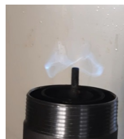
"Crown" flame when burning acetone
